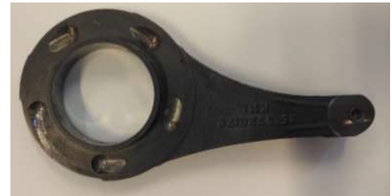
Ball ramp inner side
